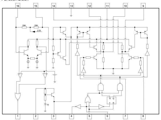
Figure 3. Function Block Diagram of XL1192A
