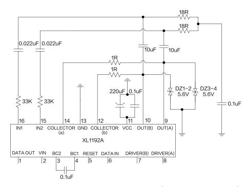
Figure 4. XL1192A Typical Application Circuit (No external transistor)
