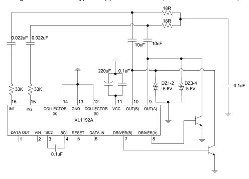
The external transistor can increase the drive
