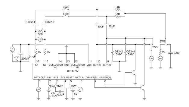
Figure 7. XL1192A Measuring Circuit (With external transistor)
