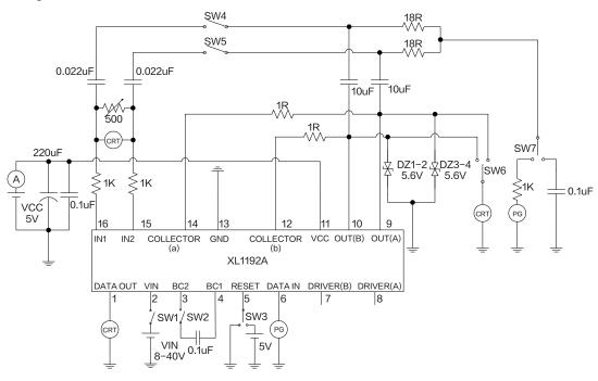
Figure 6. XL1192A Measuring Circuit (No external transistor)
